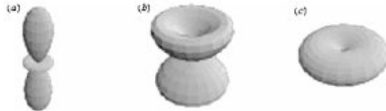
FIGURE 4. Graphical representation of spherical harmonics (a) |Y^{20}(\theta, \phi)| , (b) |Y^{21}(\theta, \phi)| , and (c) |Y^{22}(\theta, \phi)| .
